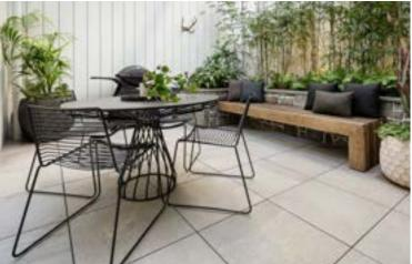
TILE SIZE: 600X600X20MM INSTALL ON QWICKBUILD WITH OUTDURE ACCESSSORIES TO HOLD THE TILES INTO PLACE
